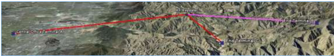
Figure 3 RF-8000E Y-Junction Repeater, 3-Hops
