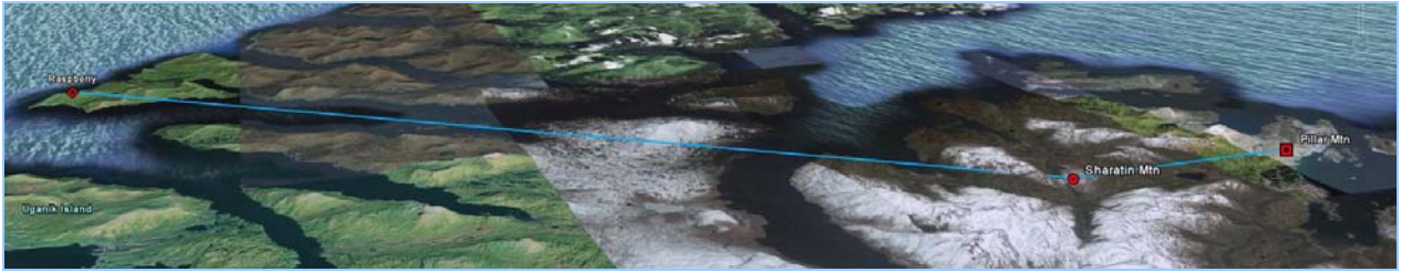
Figure 5 RF-2000E Clearing an Obstructed Path, 2-Hops
