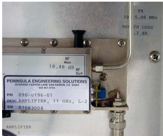
Figure 20 Power Amplifier RF MON and TX Branch Loss
