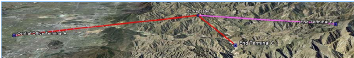
Figure 3 RF-11000E Y-Junction Repeater, 3-Hops
