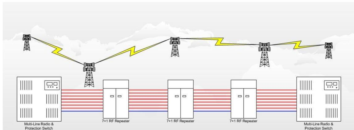
The typical upper limit in the number of tandem RF repeaters is 3 to 5. This results in 4 to 5 radio hops comprising a modulation section. Modulation sections can span 100 to 150 miles<sup>xii</sup>.
